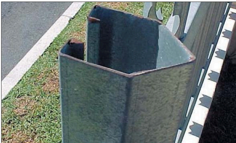
The edge protection properties provided by a zinc / aluminium coating are substantially less than that provided by a hot dip galvanized coating.
